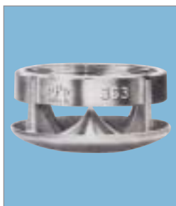
OPW-ES 363 – Cast aluminum with female threads for 2" or 6" liquid loaders used on gravity discharge lines. Available in 2" and 6".
