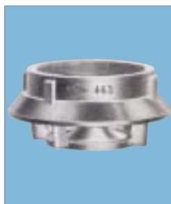
OPW-ES 463 – Cast aluminum with female threads for 3" or 4" liquid loaders. Vertical wing ribs help drop tube from rising when filling. Accelerates discharge and prevents roiling of product when used on pressure discharge line. Available in 3" and 4".
