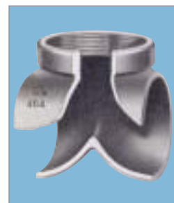
OPW-ES 464 – Cast aluminum tee with female threads. Especially designed for handling jet fuel. Prevents high velocity impingement on bottom of tank to reduce possibility of ignition of jet fuel. Available in 3" and 4".
