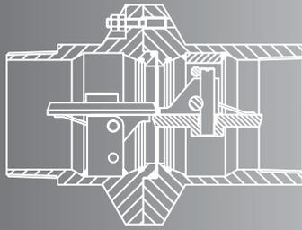
The flaps are released and allow the bias springs to rotate through a controlled arc...
