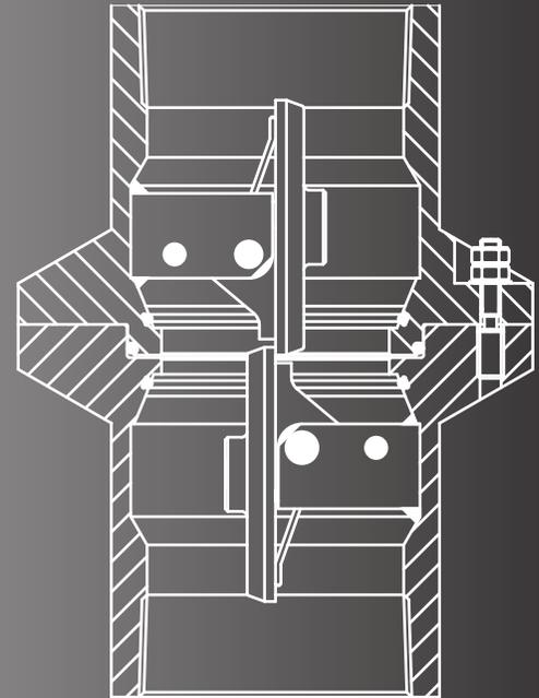
A PASSIVE SHUT OFF VALVE THAT OFFERS NO PARTIAL BREAK (no uncontrollable spillage)
