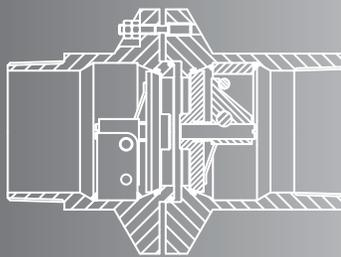
With 100% shut-off achieved, the two halves of the coupling then part completely.
