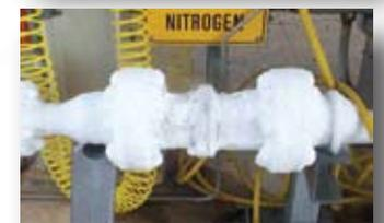
Cryogenic Passive Shut-Off Valve
