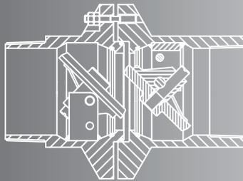
... until they have moved through 90°, where they snap onto their seats prior to the coupling fully parting.
