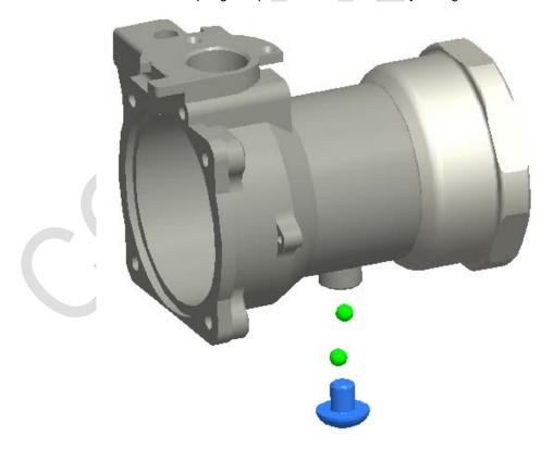
Remove ball plugs and rotate swivel and body so bearings can fall out (1 and 2 inch unit shown)
