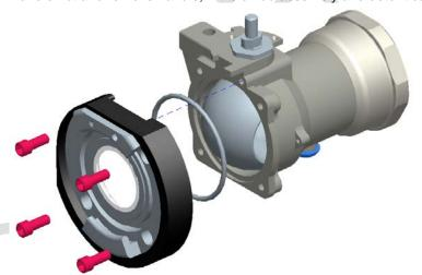
• Loosen flange bolts and remove flange / ball seal assembly and flange seal
