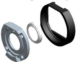
• Pop ball seal (16) out of flange, remove flange from rubber bumper
