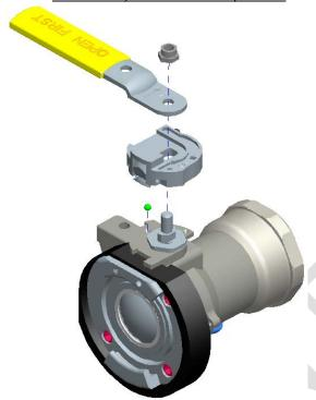
• Loosen handle nut and remove handle, handle hub assembly and detent ball
