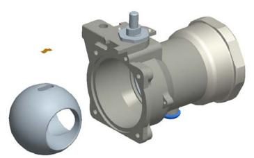
• Rotate ball out of socket, be sure to secure conductivity spring located in blind slot
