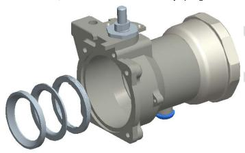
Pull ball seal along with washer and spring out of body
