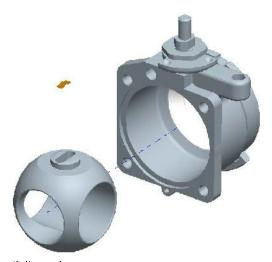
• Remove ball and conductivity spring
