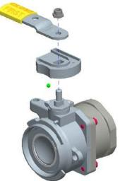
• Loosen handle nut and remove handle, handle hub assembly and detent ball
