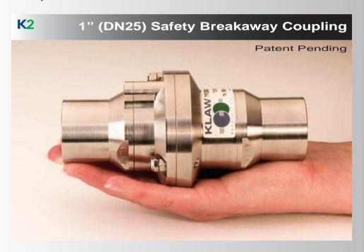
**K2** is the all NEW 1" (DN25) Safety Breakaway Coupling, it utilises the world renowned KLAW Flip-Flap mechanism, which offers many distinct advantages including, low pressure drop, light weight compact design, NO partial break with uncontrollable spillage.
